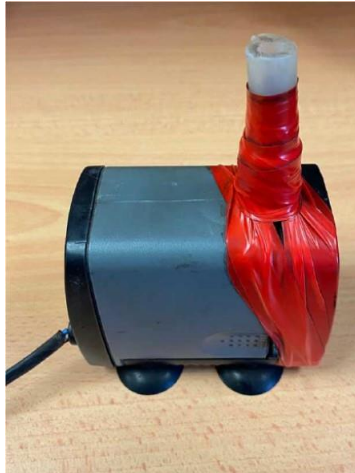
The fish tank style pump with damaged lead
