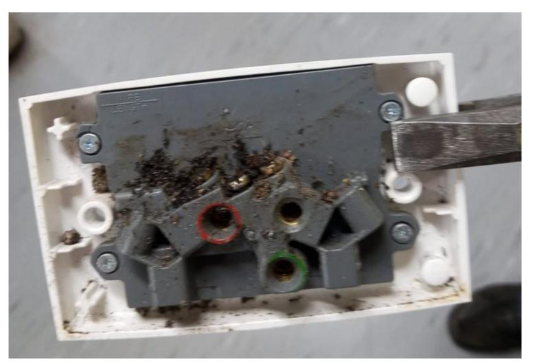
A view of the back of the outlet with the termite debris becoming like mud across the terminals
