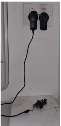
How the unit owner found the power supply. Note the burn mark above the right hand plug in the outlet, the unit on the shelf and the splatter marks on the white shelf The power supply on the left was unaffected.
