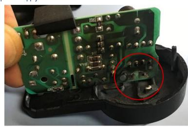
How the power supply was mounted inside the unit. Note the burn mark on the bottom of the card where the 240V ac cables would have been, these cables were completely disintegrated.
