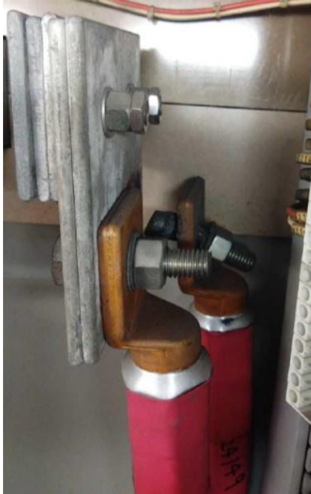
The bolted connection clearing open circuited from the busbar by the weigh of the cable and head of the bolt melting off
