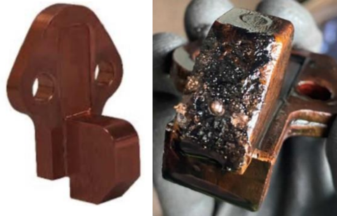
A new and the used arcing (or sacrificial) contact which is used to suppress any arcing during switching
