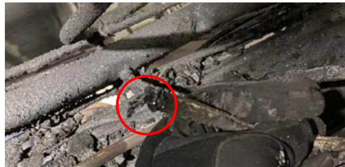
The two severed ends of the emergency stop cable
