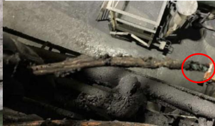
The two severed ends of the emergency stop cable
