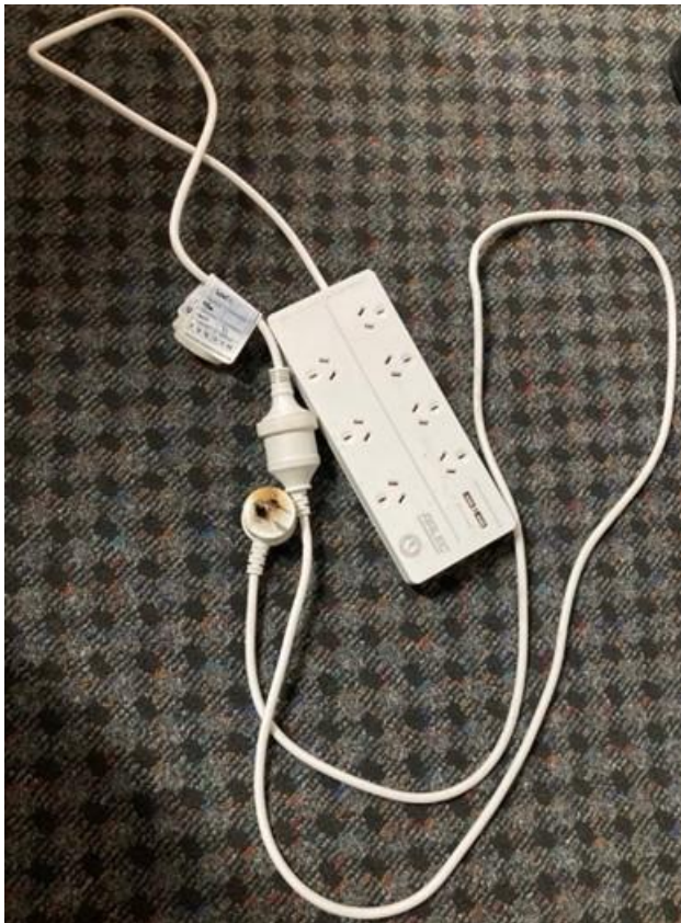
The 7-way outlet board with the short extension lead, which does not have overload protection
