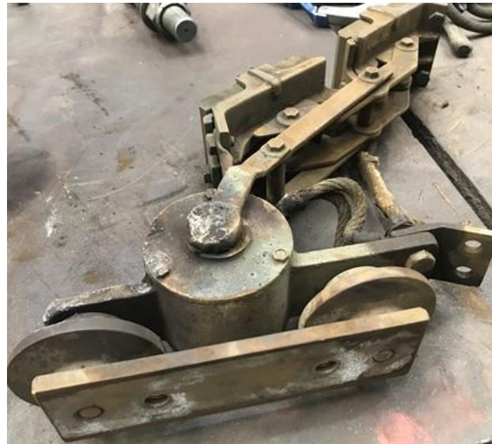
The bottom phase collector shoe and arc marks
