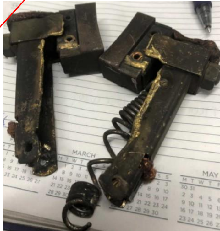
The damaged brush arms with the failed spring
