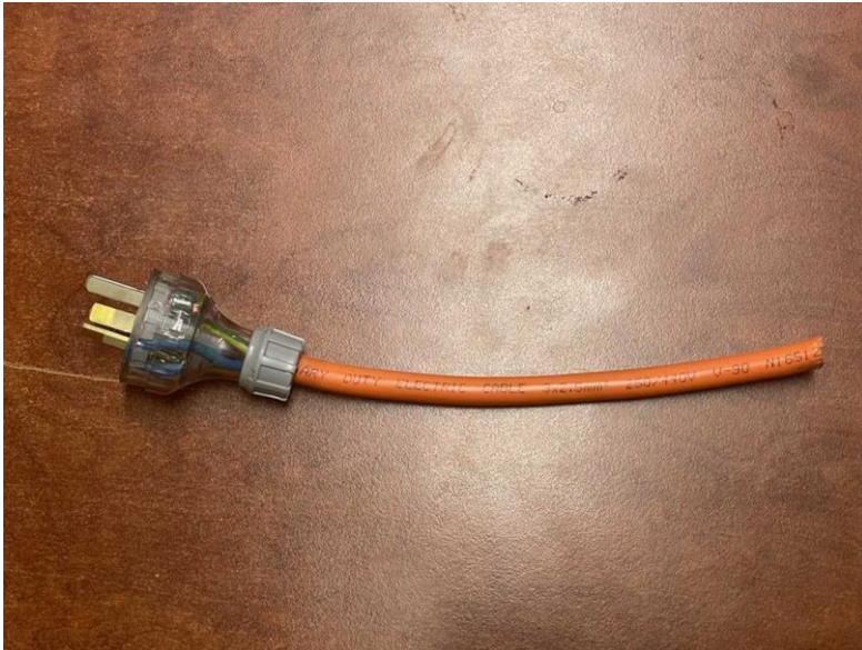
240 Volt plug and severed cable
