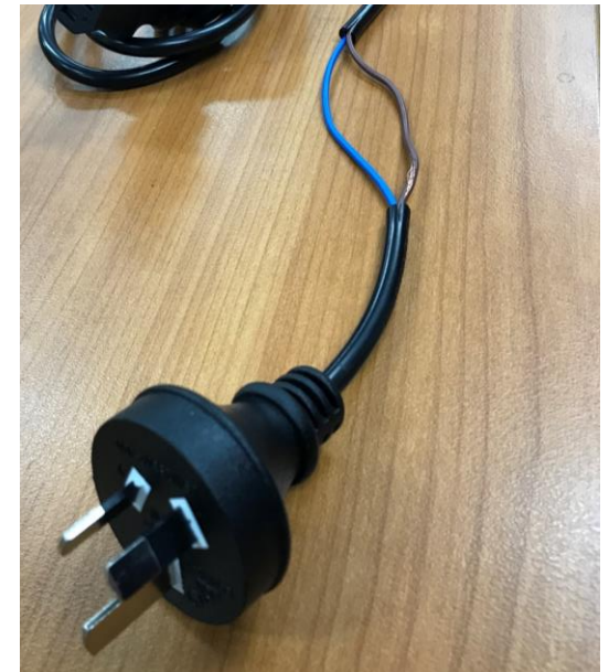
Only 2 wires in cable, no Earth conductor
