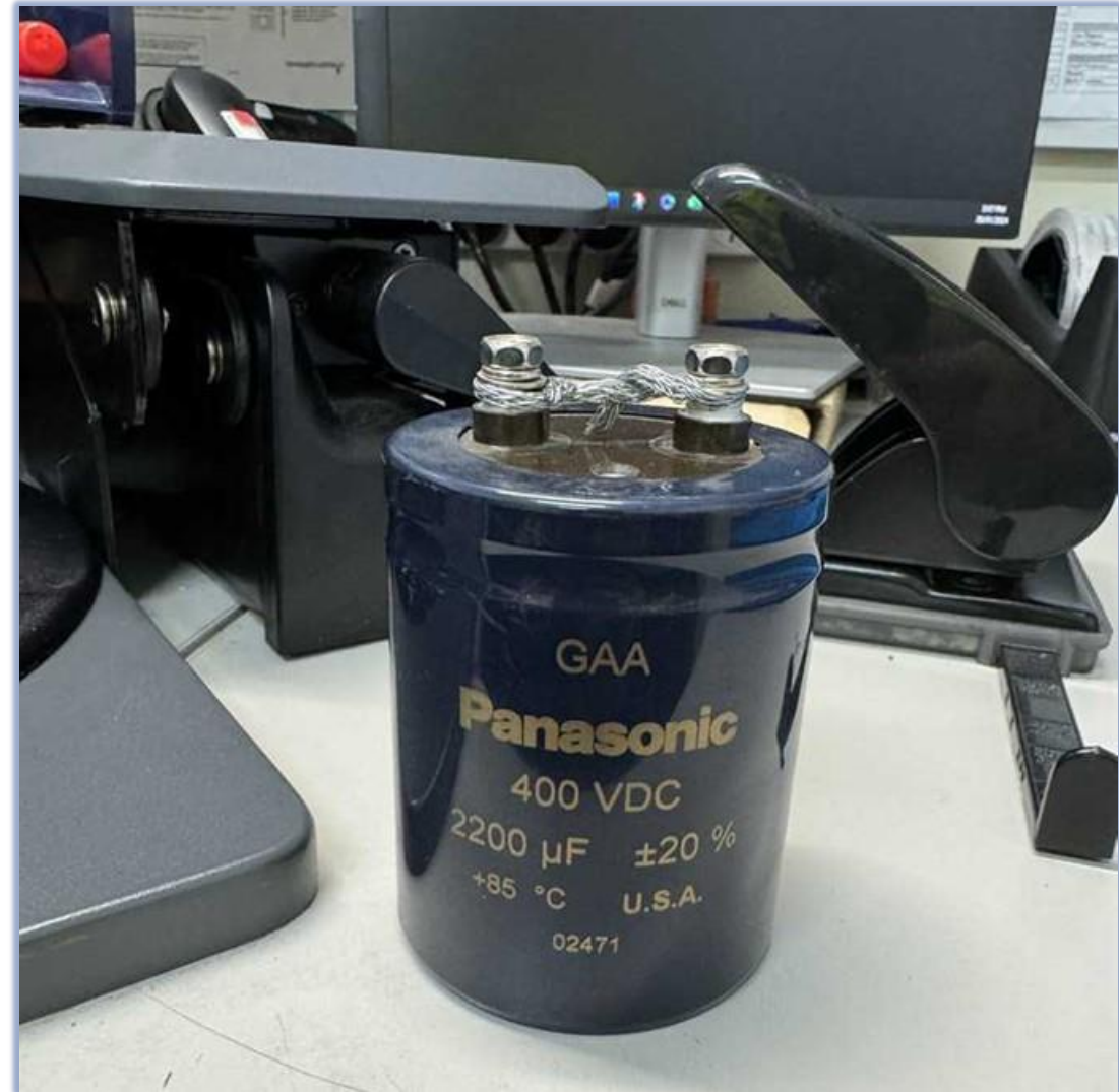
Capacitor with terminals shorted for storage
