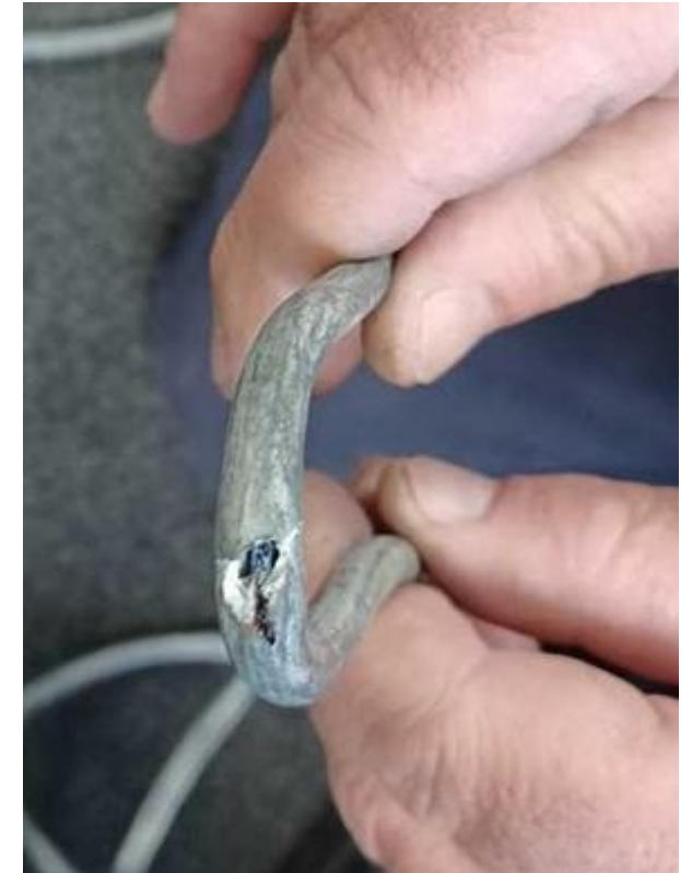
Damaged Vacuum Power Lead
