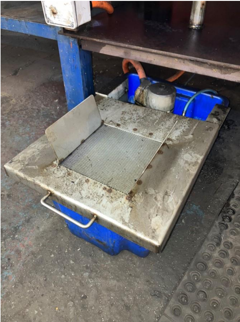
Modifications - coolant tub, 415-volt pump, bracket & tray
